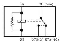
Relay Pin 87a has power in the de-energized state until the coil pulls the switch to the opposite pole at Pin 87.
