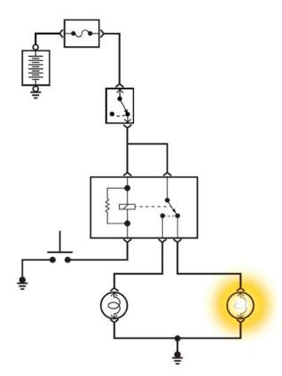
If two lighting circuits are powered by the relay circuit, voltage to the lights will toggle and the bulbs will illuminate OFF/ON based on the state of the relay.
