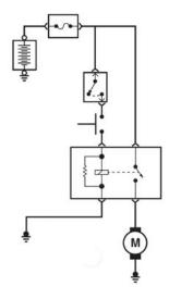
Energizing the starter relay begins the process of providing the electrical-to-mechanical connection to start the engine.
