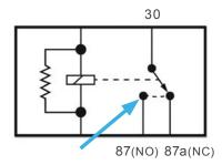
Testing between Pin 30 and Pin 87 (Pin 87a if applicable) will let you know if current can pass through with low resistance. If resistance is high, it will impede the flow of current to the load.
