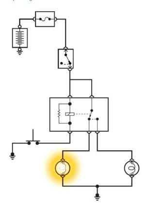
The low and high beam headlamp circuits use relays in a similar manner.
